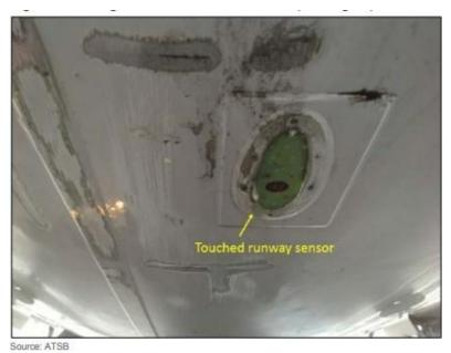
Figure 2 - Damage to tail section VH-QOS (looking aft)
